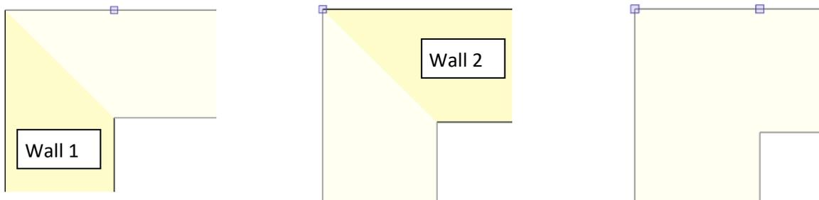
Note wall 1 end point, and wall 2 end points do not coincide, both highlighted and shown on 2D or 3D. Although the walls seem to attach, as the wall end points are not on top of each other DAISY™ will see a gap in the walls and reject the design.
